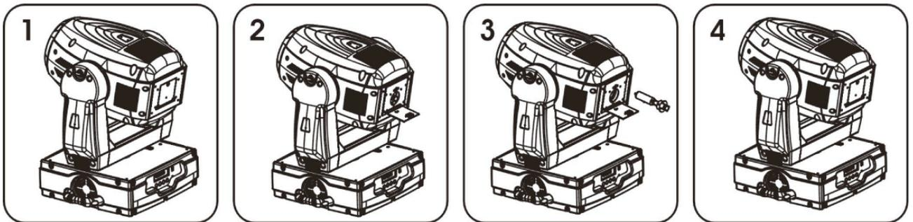
1. Set the fixture on a flat surface and turn the ¼" turn locking screw counter-clockwise until they unsecured.
