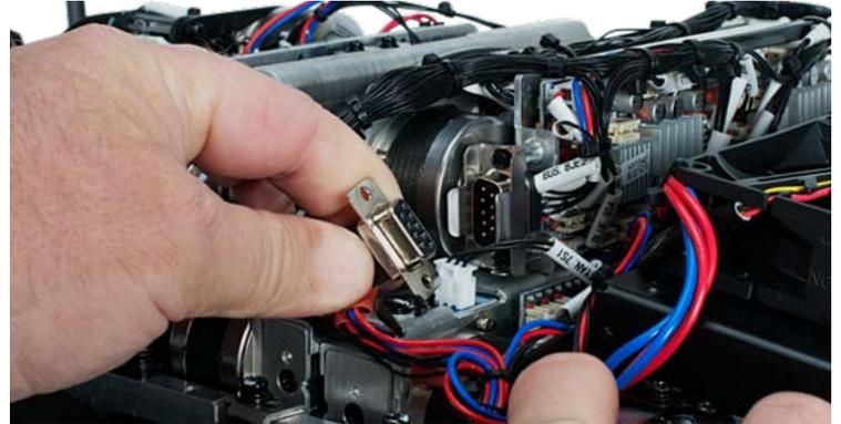
5. Locate the 9-pin connector and carefully unplug it from its socket. DO NOT USE FORCE TO REMOVE!
