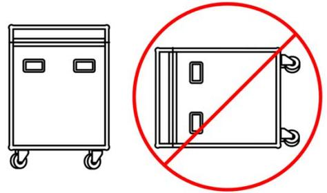
DO NOT Tip the case over, and avoid all shocks and rough handling, especially “tipping”, the practice of tipping the fixture-case over to its side and onto a hard surface. The case must ride on its wheels so that the fixture-head remains horizontal during transportation.
