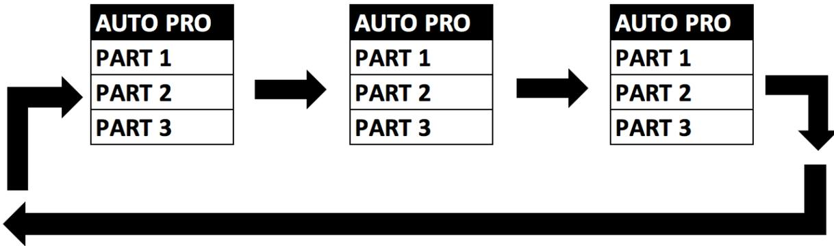
The Secondary unit receives data from the Primary unit according to the group which the Secondary unit was assigned to. If e.g. a Secondary unit is set to “Secondary 1” in the menu “Set to Secondary”, the Primary unit sends “Auto Program Part 1” to the Secondary unit. If set to “Secondary 2”, the Secondary unit receives “Auto Program Part 2”.
