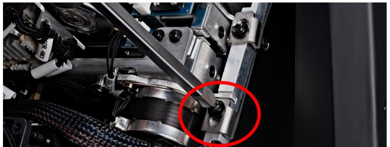
3. The GOBO Wheel module is secured to the fixture frame rail with (4x) sliding slotted brackets. To remove the module, loosen the (4x) Philips-head screws just enough (do not remove them) to allow the slotted brackets to slide down.
