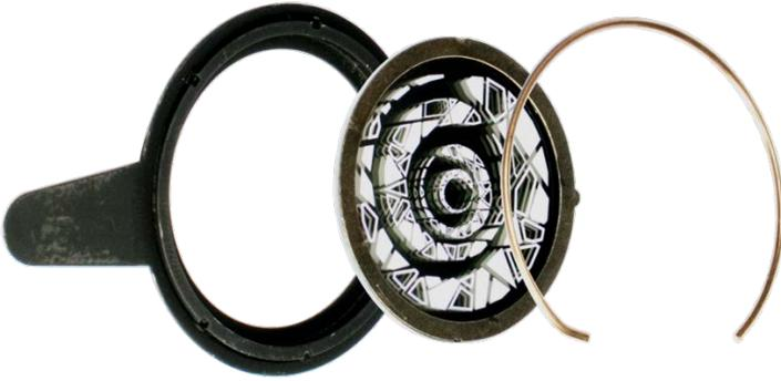
12. Locate the tab of the retaining spring. Using a precision pick (or similar tool), carefully press the retaining spring inward to relieve the tension. Remove the retaining spring and carefully separate the GOBO from the GOBO Holder. Lastly, remove the flat washer attached to the removed GOBO and attach it to the desired replacement GOBO. Install the replacement Static GOBO following the steps above in reverse order.
