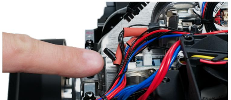
4. The wire harnesses connected to the GOBO Wheel module are secured with a flexible metal stay. Unbend this metal stay to ungroup the wires connected to the GOBO Wheel module.
