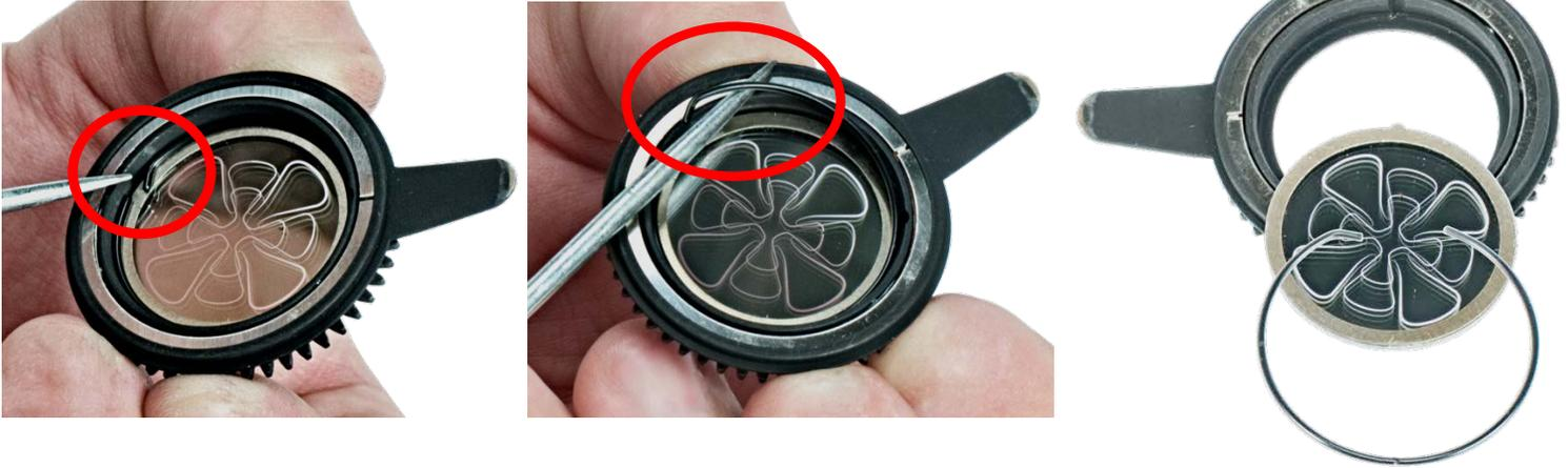
10. Locate the tab of the retaining spring. Using a precision pick (or similar tool), carefully press the retaining spring inward to relieve the tension. Remove the retaining spring and carefully separate the GOBO from the GOBO Holder. Lastly, remove the flat washer attached to the removed GOBO and attach it to the desired replacement GOBO. Install the replacement Rotating GOBO following the steps above in reverse order.
