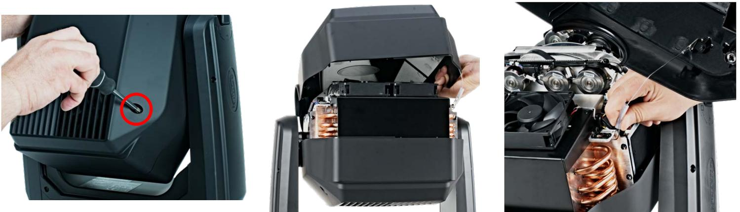
2. Loosen (2x) ¼-turn Phillips-head screws on top and bottom covers. (screws integrated into covers - cannot be removed)
