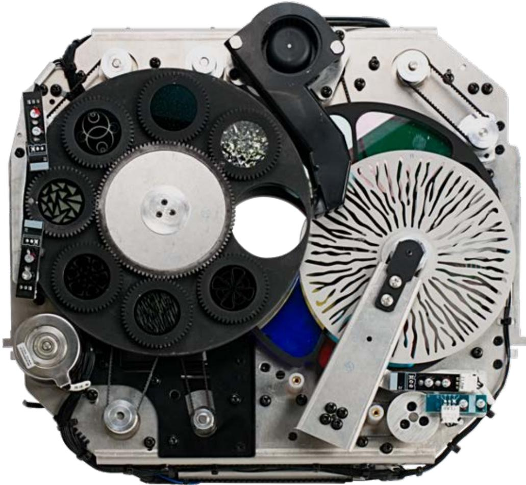
8. Slide the GOBO Wheel module completely out and away from the fixture. Carefully place the module on a stable flat surface in an INDOOR DUST FREE location.
