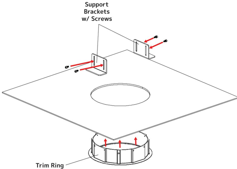
1. Open an 8.5-inch diameter hole in the desired ceiling panel. Insert the trim ring through the hole, and secure in place with the support brackets and screws.
