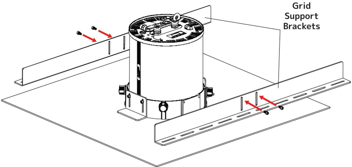
3. Attach the grid support brackets to the trim ring using the included screws.
