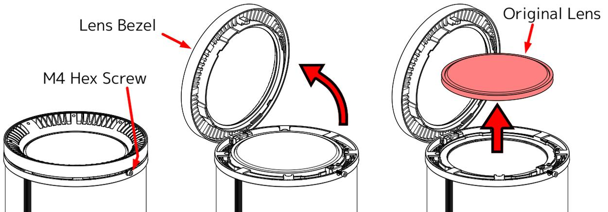
2. Insert Optional Lens, ensuring that it is positioned correctly to fit into the notch recesses, then close and secure lens bezel with screw.
