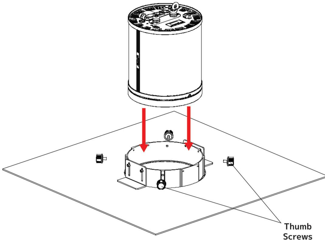
2. Lower the lighting fixture into the trim ring from above, then secure in place by inserting and tightening the four (4) thumb screws.
