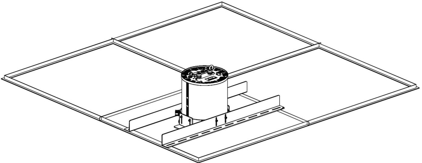
4. Install the entire assembly back into the ceiling at the desired location, making sure that the ends of the grid support brackets are resting firmly on the support grid for the ceiling. Secure the grid support brackets in place using the appropriate hardware.
