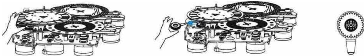
Locate the (1x) screw on the side of the Pattern Bracket Assembly
