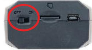
1. With the software update stored on the MICRO SD card, insert the SD card into the slot located at the bottom of the E-Loader III.
