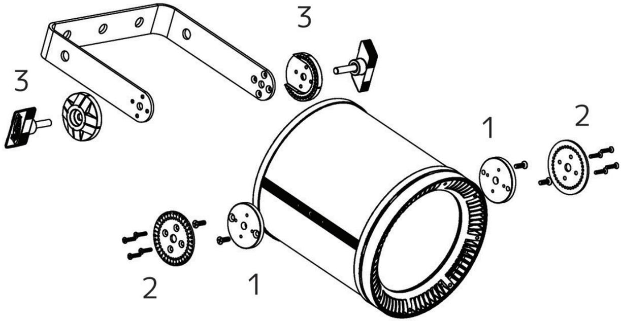
1. Attach the two (2) yoke spacer discs to the fixture with two (2) screws each.
