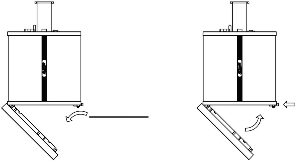
1. Loosen screw on the side of lens bezel to open/release, as shown in the image on the left.
