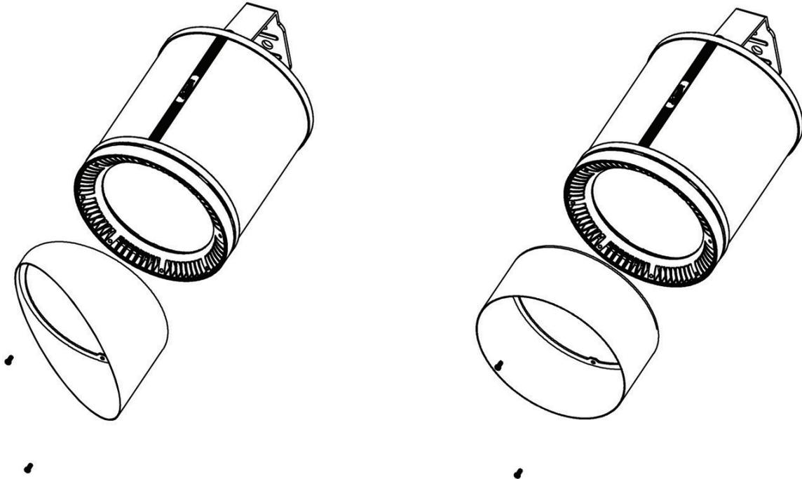
To install either snoot kit, align the desired snoot with the lens bezel of the fixture, and secure the snoot in place with two (2) screws).
