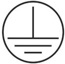
**PROTECTION CLASS 1 - FIXTURE MUST BE PROPERLY GROUNDED.**
