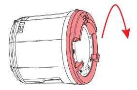
Insert the mounting tabs on the Bowens lens into the matching slots on the Bowens adapter, then twist to secure in place.
