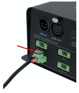
Now insert the wire leads from the fixture into the wire terminals of the Phoenix connector, making sure that the bare wire lead ends have been fitted with wire end sheaths. Tighten the two screws above the wire terminals, as shown in the image at above right, to secure the wire leads in the Phoenix connector.
