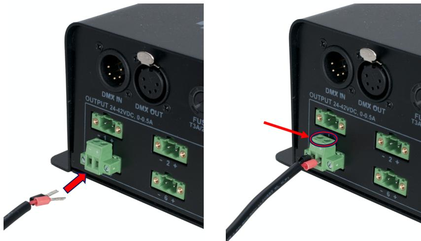
Now insert the wire leads from the fixture into the wire terminals of the Phoenix connector, making sure that the bare wire lead ends have been fitted with wire end sheaths. Tighten the two screws above the wire terminals, as shown in the image at above right, to secure the wire leads in the Phoenix connector.
