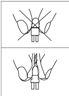
**DISCHARGE LAMP WARNING:** This fixture is fitted with a discharge lamp, which is highly susceptible to damage if improperly handled. Never touch the lamp with your bare hands, as the oil from your hands will shorten lamp life. Also, never move the fixture until the lamps have had ample time to cool. Remember, lamps are not covered under warranty conditions.
