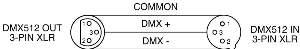
*Be sure to follow the above figure when making your own cables. Do not use the ground lug on the XLR connector. Do not connect the cable's shield conductor to the ground lug or allow the shield conductor to come in contact with the XLR's outer casing. Grounding the shield could cause a short circuit and erratic behavior.*
