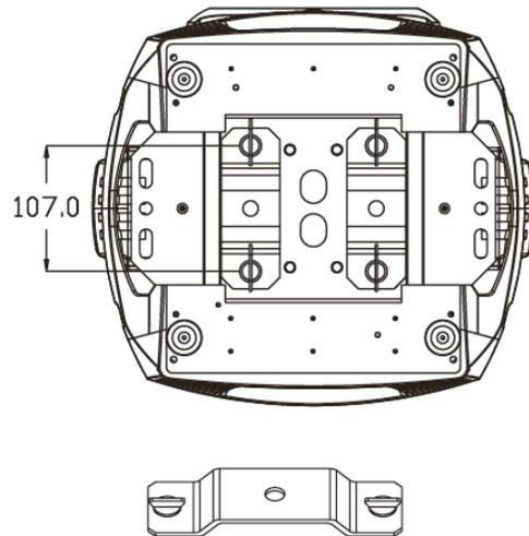
Note: Please add 76.5mm to the total height of the fixture when using the included Omega-Clamp
