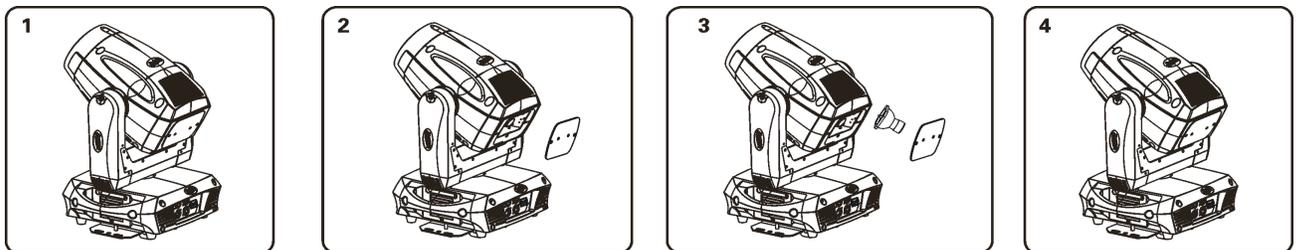
1. Set the fixture on a flat surface and remove the two screws marked “A” and “B”.
