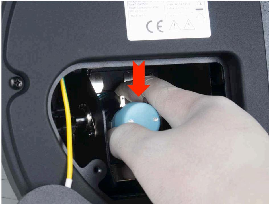
5. Once lamp is released, grab the lamp base with your thumb and index finger and gently pull the lamp **OUT** towards and **AWAY** from the fixture.
