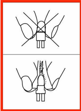
This fixture is fitted with a DISCHARGE LAMP, which is highly susceptible to damage if improperly handled. NEVER touch the lamp with your bare hands, as the oil from your hands will shorten the life of the lamp. Also, NEVER move the fixture until the lamp has had ample time to cool. Lamps are NOT covered under warranty conditions.
