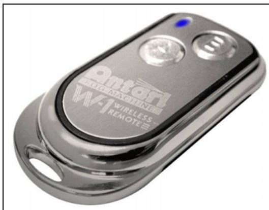
With the transmitter it is possible to output via radio over a distance of up to 50 meters. The transmitter is compatible to any receiver of SW-250 and can control an unlimited number of machines in parallel. Press the button "A", to output. As control, the LED on the transmitter is lit. To stop the output, press the button "B".
