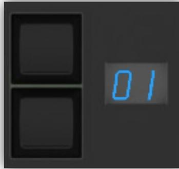
There are 2 separate sets of page control buttons, one for the Playback Faders and another for the Matrix buttons. Paging essentially gives you additional virtual sets of faders and matrix buttons to work with. Paging can be controlled by your lighting software or by the **MIDICON-2™** controller via MIDI channel paging. If your software can control the paging you can have up to 99 pages to work with.
