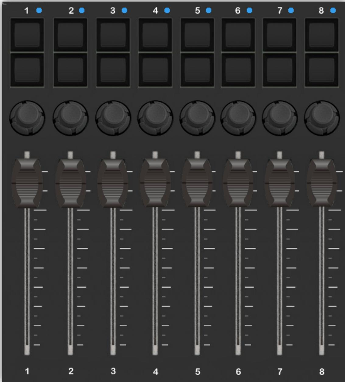
The playback section was designed to take advantage of the playback features in most lighting software programs where a playback fader and some associated buttons are used. There are two buttons, a small rotary encoder and a red/blue bi-color LED above each fader. The function of each of these will vary depending on the software that you are using.
